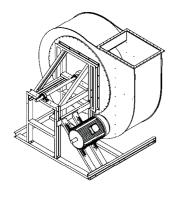
3. Screw housing to fan rear panel.
